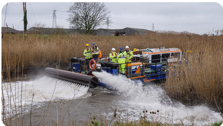
(Pictured: Van Oord's water injection dredging vessel "Borr" in display mode with water injection bars raised, during a short trial near Moorland in January 2020. The bars are usually submerged)
